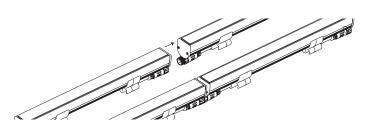
**3e** When properly installed, NANO WD Rigid connection should result in little to no gap between fixture end caps.
