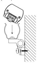
$\mathbf{2c}$  When one corner is inside the clip, turn fixture to "roll" the rest into the clip.
