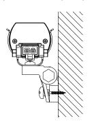
**2e** Recommended location of the clips, Length of fixture is not relevant.
