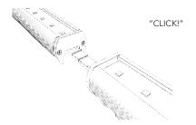
**3e** When properly installed, NANO WD Rigid connection should result in little to no gap between fixture end caps.
