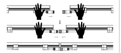
${f 3e}$  When properly installed, NANO WD Rigid connection should result in little to no gap between fixture end caps.
