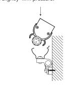
**2c** When one corner is inside the clip, turn fixture to "roll" the rest into the clip.
