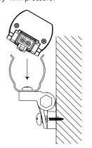
**2c** When one corner is inside the clip, turn fixture to "roll" the rest into the clip.
