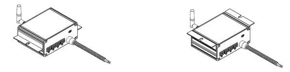
Note: Mounting brackets can be configured in a variety of positions.
