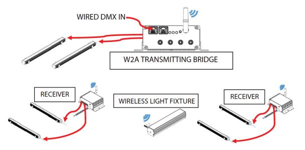
3. Wireless DMX input to wired output (A2W Bridge Mode)
