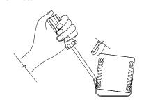
**7c** Once released from one notch, fixture can be fully removed.
