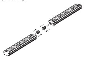
**4c** Push together and then twist until completely connected and
