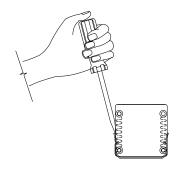
**7b** While holding the fixture with your other hand, pull back on screwdriver to release from notch.
