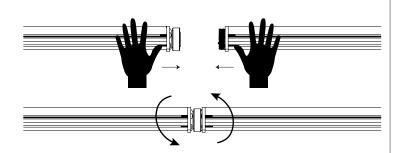
**3e** Screw fixtures together at the connection points to ensure no damage is done to the fixtures. #2 screw provided by Boca.
