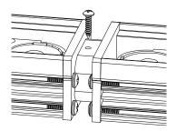
**IMPORTANT NOTE:** Not screwing fixtures together represents an incomplete install and voids the warranty if any fixtures are damaged as a result of improper installation.
