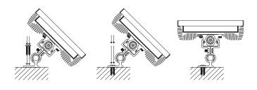
**1b** Loosen center hinge pin and adjust angle of fixture to focus required. Tighten pin to hold the focus.
