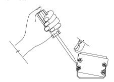
**7c** Once released from one notch, fixture can be fully removed.
