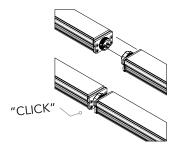
**IMPORTANT NOTE:** Not screwing fixtures together represents an incomplete install and voids the warranty if any fixtures are damaged as a result of improper installation.
