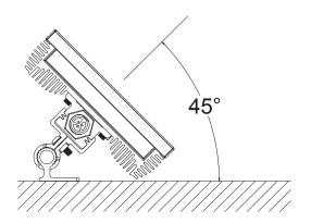
\*SBL-Mix Fixtures will ship with swivel mounting brackets attached to fixture. (Two swivels per fixture) Clips are installed opposite side of fixture cables to allow maximum swivel ability.
