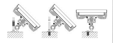
**1b** Loosen center hinge pin and adjust angle of fixture to focus required. Tighten pin to hold the focus.
