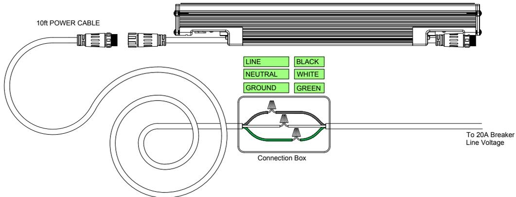
**7. CONNECT FIXTURES TO DIMMING SYSTEM**
