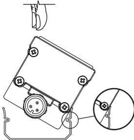
**2b** Fixture will pivot on notch as it is pushed down.
