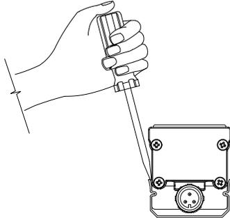
**8b** While holding fixture with other hand, pull back on screwdriver to release from notch.
