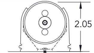
FIXED TUBE- FIXTURE CAN ROTATE IN TUBE
