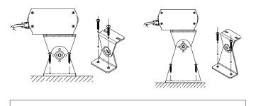
\* HPFB Fixtures will ship with swivel mounting brackets attached to fixture. (Two swivels per fixture) Clips are installed opposite side of fixture cables to allow maximum swivel ability.
