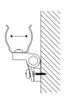
**2b** Push Fixture down into the clip at an angle with slightly firm pressure.
