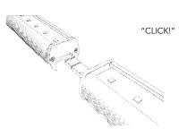
**3e** When properly installed, NANOLUME connection should result in a little gap between fixture end caps.
