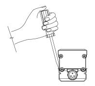
**6b** While holding fixture with other hand, pull back on screwdriver to release from notch.
