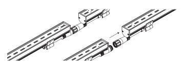
3e When properly installed, NANO WD Rigid connection should result in little to no gap between fixture end caps.
