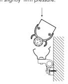
**2c** When one corner is inside the clip, turn fixture to "roll" the rest into the clip.
